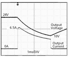
Peak load 6.5A (resistive load) for 5ms Output voltage dips from 24V to 10V.
