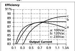
Fig. 8-3 **Efficiency vs. input voltage at 24V, 1.3A, typ.**
