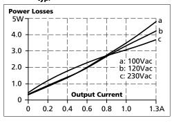
Fig. 8-4 Losses vs. input voltage at 24V, 1.3A, typ.
