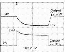
Peak load 2.6A (resistive load) for 50ms Output voltage dips from 24V to 16V.
