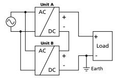
orientations other than the standard mounting orientation (input terminals on the bottom and output terminals on top of the unit). Be ware that leakage current, EMI, inrush current and harmonics will increase when using multiple power supplies series.
