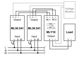
more. This can only be avoided by utilizing decoupling diodes which are included in the redundancy module MLY10.241.
