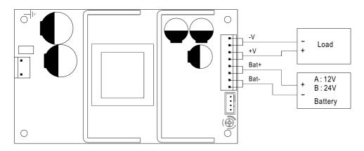
Fig 1.1 Suggested system connection
