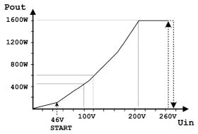
Output power / input voltage derating curve
