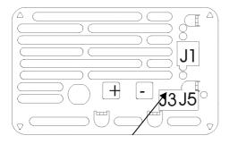
The temp.comp cable enables the charger to adjust the output voltage in accordance with battery voltage and temperature fluctuations
